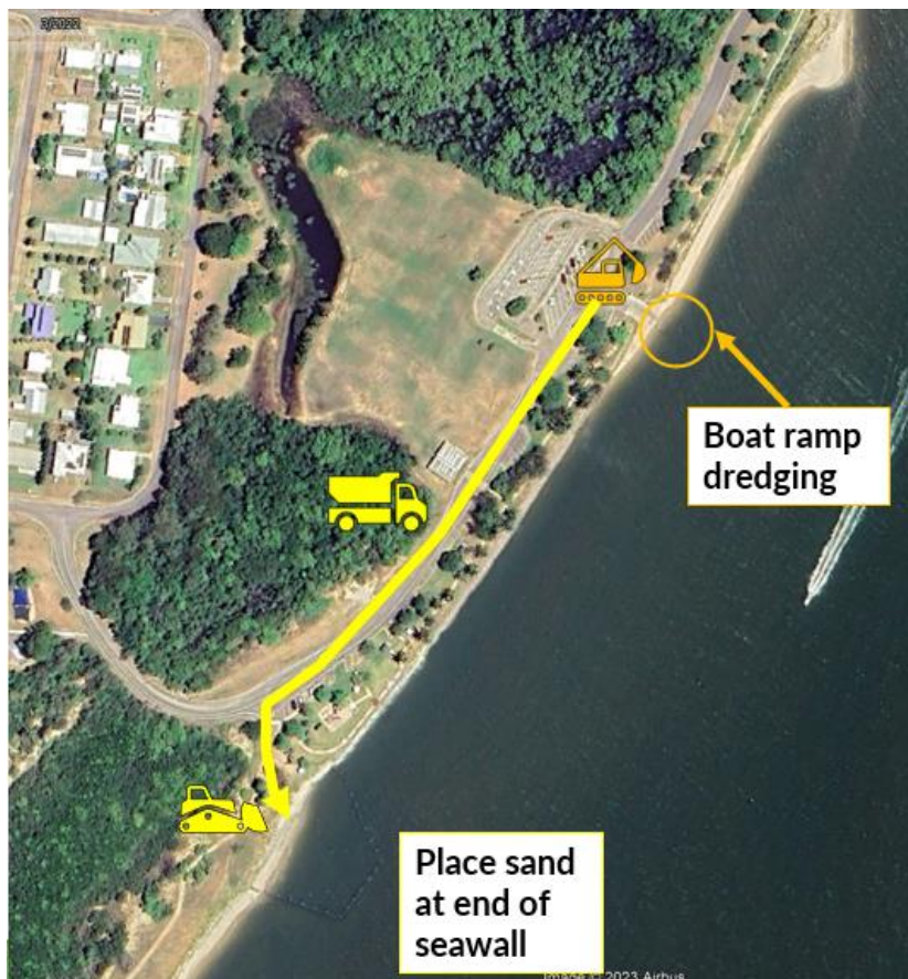
Figure 6-17 Indicative arrangement of dredge material reuse at Taylors Beach
